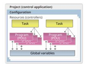
Applications can be developed in project units. A project consists of one or more configurations (programs) running on several different resources (controllers). Multiple tasks are allowed to run on each controller.
